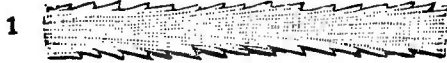
1. A fibre of long Merino, viewed as a transparent object by the microscope.
